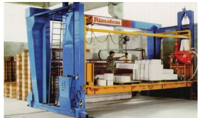
Figure 3. Partially automated masonry element prefabrication.
