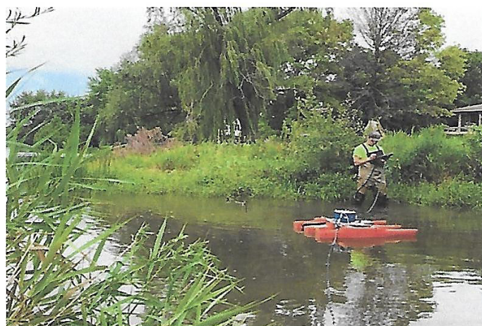
Figure 2. ADCP streamflow measurement.
