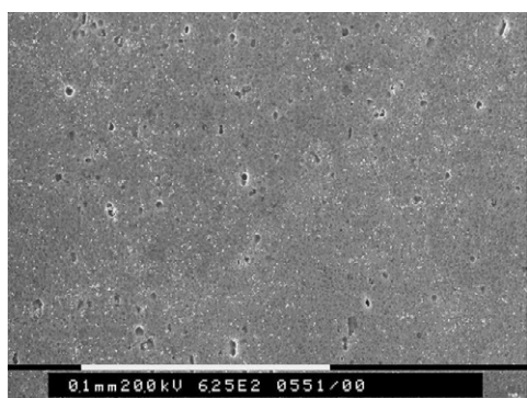
Figure 4: A Typical SEM micrograph showing the distribution of particles present in the as received sheets.
