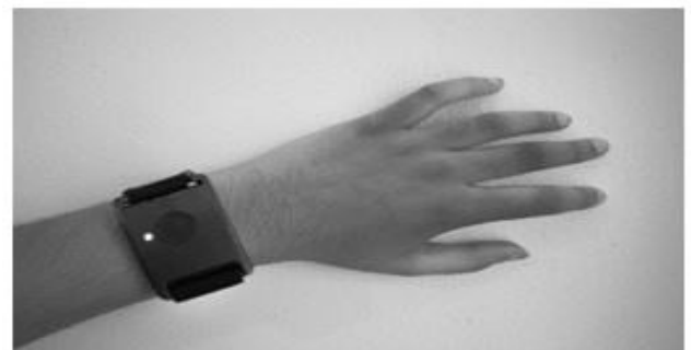
Figure 1. Wrist watch. Wearable device for epileptic patients which gives alarm during pre-ictal state.
