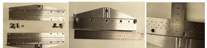
Figure 1. Clamp head for fabric tensile test.
