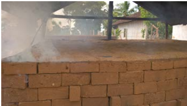
Figure 4: Traditional firing method of clay bricks.
