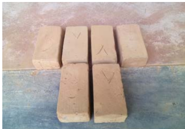
Figure 3: Sri Lankan standard brick size: 20.5 cm × 9.5 cm × 7.5 cm.
