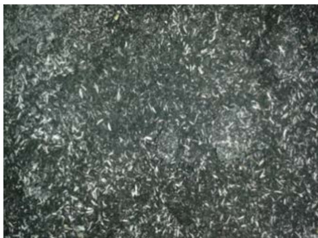
Figure 2: Coarse ashes with large particle size were found in the grey-whitish ash obtained after burning at 600°C to 900°C.
