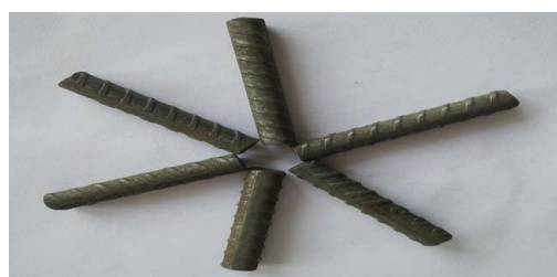
Figure 4: Steel embedded in concrete with 0.5% of hexamine after 180 days exposure.
