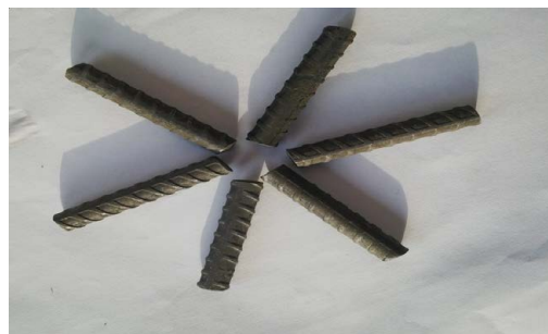
Figure 3: Steel embedded in concrete with 0.5% of calcium nitrite after 90 days exposure.
