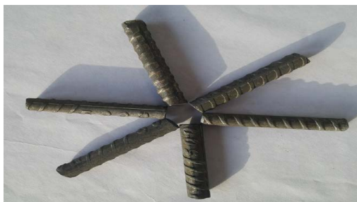
Figure 1: Shows corrosion of steel bar embedded in the blank sample after 90 days of exposure.
