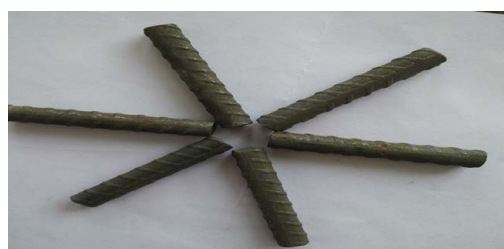
Figure 5: Steel embedded in concrete with 0.5% of calcium nitrite after 180 days exposure.
