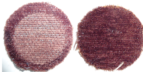
Figure 3: A specimen before and after friction test.
