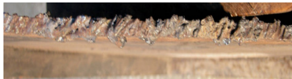
Figure 16: The control gas cut tool marks as sent by forwarding authority.
