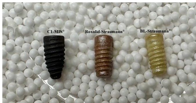
Figure 2. Enlarged photograph of the 3 groups of dental implants, after incineration. The C1-MIS® implant turned black, the Roxolid-Straumann® implant turned pink and the BL-Straumann® implant turned yellow.
