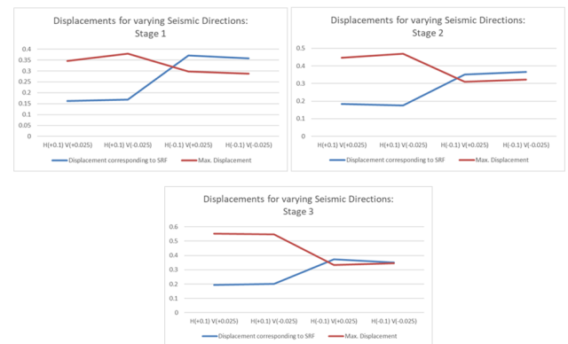
Figure 6. Displacement for varying seismic directions stages 1-3.
