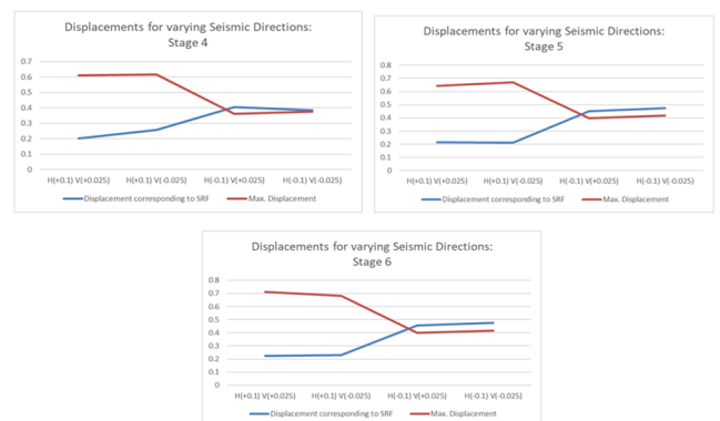
Figure 7. Displacement for varying seismic directions stages 4-6.
