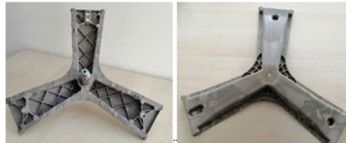
Figure 10. Injection moulded short fiber glass reinforced polyamide composite drum
