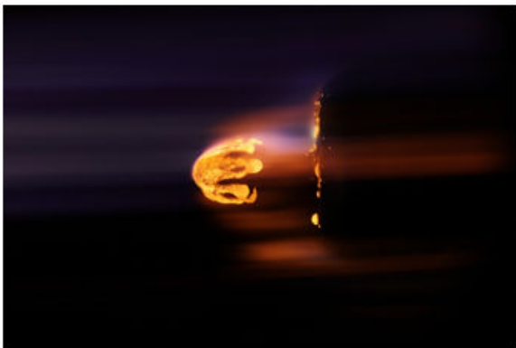
Figure 7: The simulated ablation of a chondritic meteorite at the probe of the plasma wind tunnel (image by the High Enthalpy Flow Diagnostics Group, IRS).
