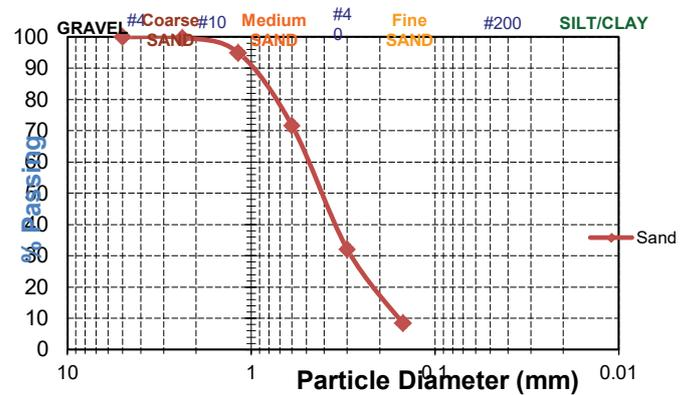
Figure 6. Particle size distribution of river sand.
