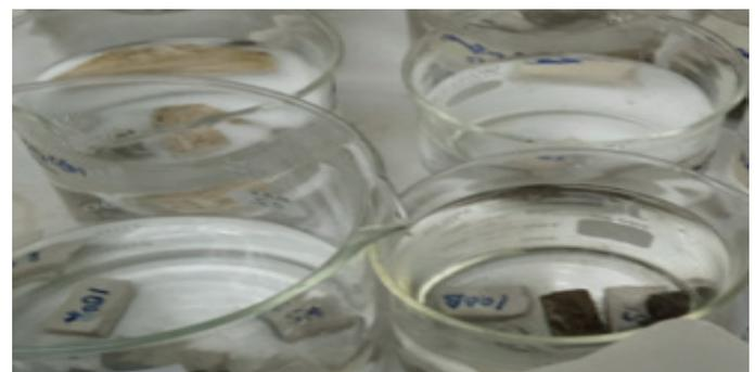
**Figure 11.** Sample soaked in different chemical for 7 days.
