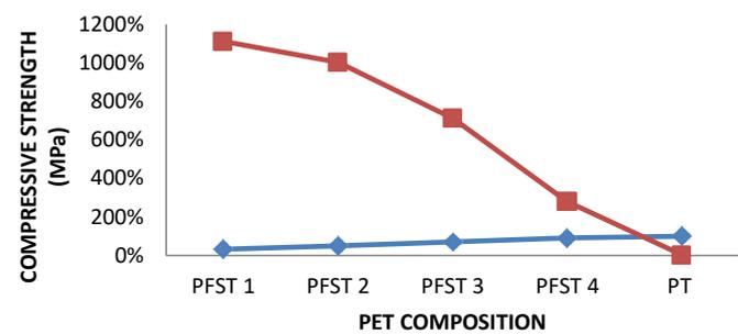
**Figure 9.** Average compressive strength values of the samples.
