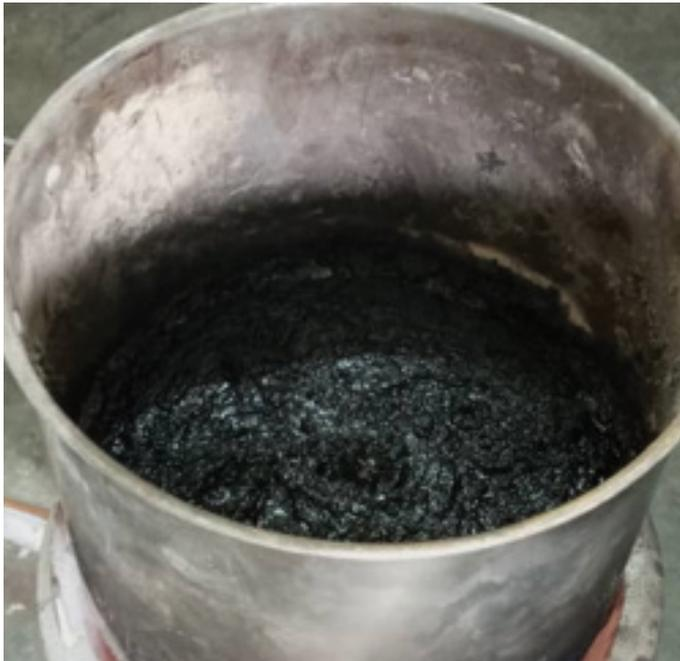
Figure 4. Melted PET mixed with sand and fly ash.
