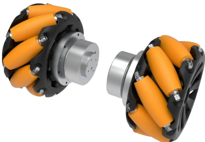
Figure 3. Mecanum wheel, a conventional wheel with a series of rollers attached to its circumference with an axis of rotation at 45° to the plane of the wheel in a plane parallel to the axis of rotation of the wheel.
